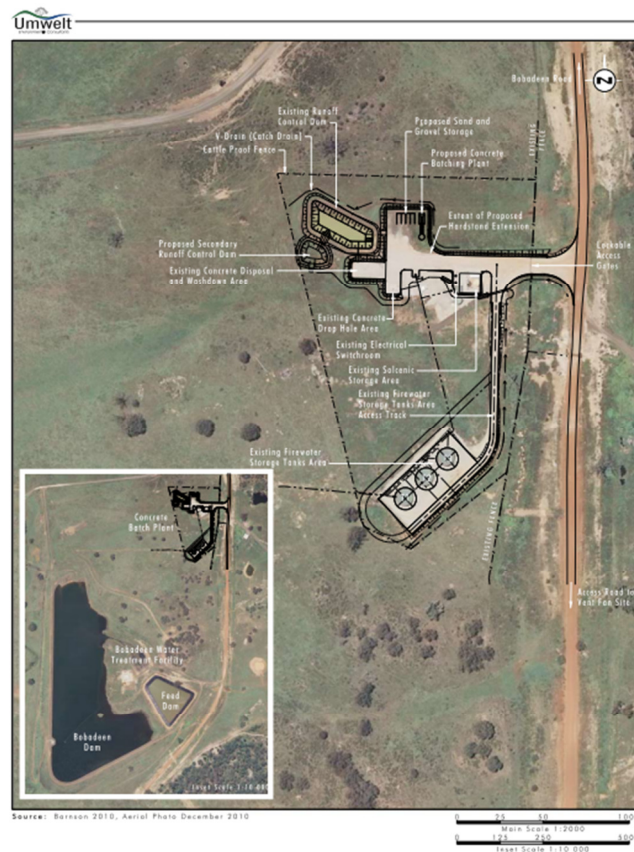
Figure 1 Proposed Concrete Batching Plant Site Layout
