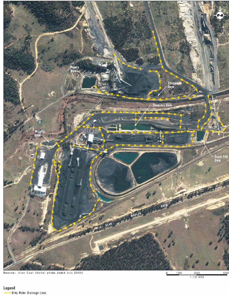
Figure 1: Coal Stockpile Run-off Diagram
