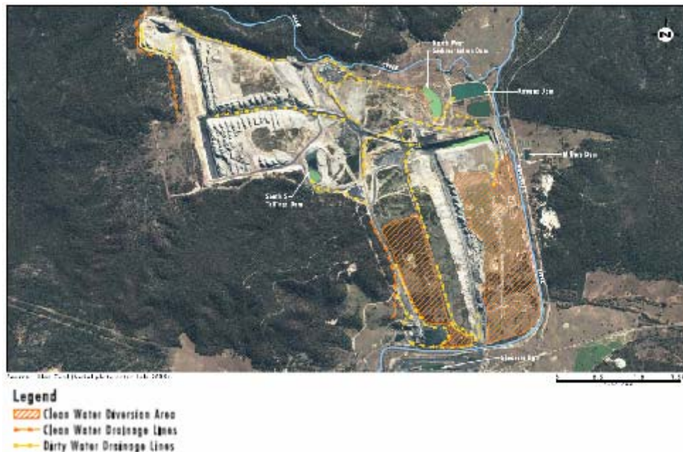
Figure 2: Diversion and Flow Paths for Water System
